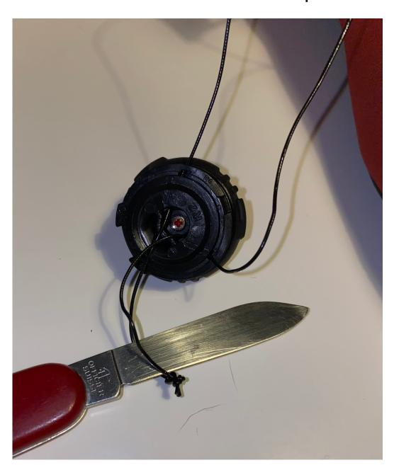
4: Secure the cable with a double knot. Cut the excess cable
