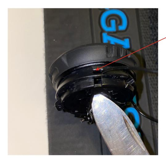
3: Insert the stainless cables into the holes as showed in the picture
